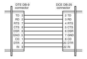
Figure F-2. 9-pin to 25-pin RS-232 cable.
